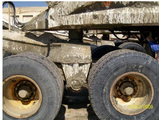
Photograph 2: coupler structure between wet haul trailers or of the hitch turret
